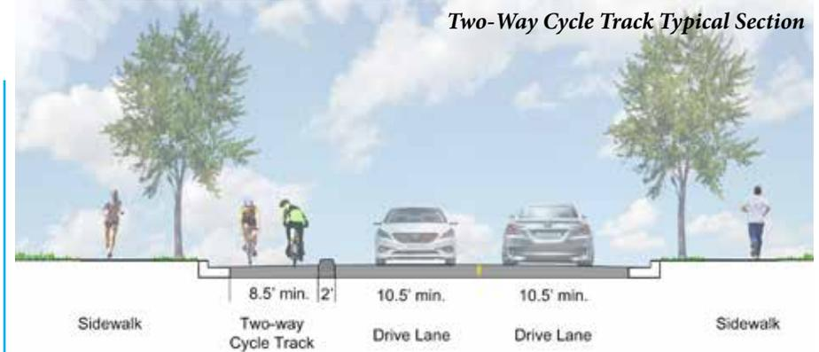
motor traffic by raised medians, on-street parking, or bollards. By separating cyclists from motor traffic, cycle tracks can offer a higher level of security than bike lanes and are attractive to a wider spectrum of the public.
