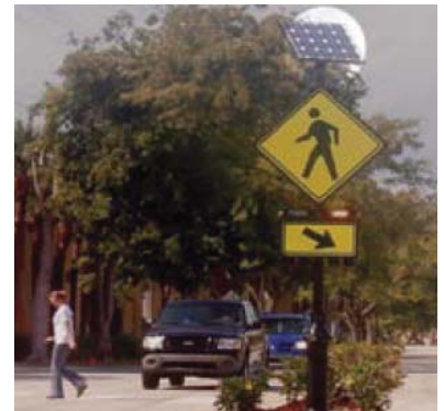
Activated, solar-powered RRFB at an unsignalized intersection flash using an irregular flash pattern (Source: FHWA)
