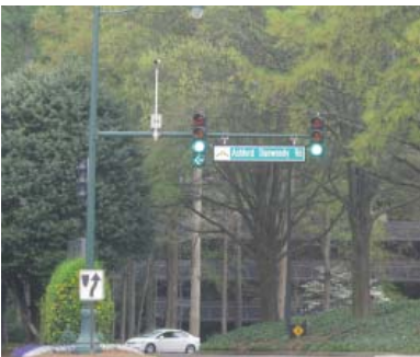
Decorative mast arm with internally illuminated street name sign
